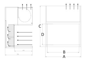
The above drawing illustrates a standard unit., with rear acess HEPA removal. The arrows show the directions of airflow through the unit. The letters referenced in the Darwing and tables refer to:
