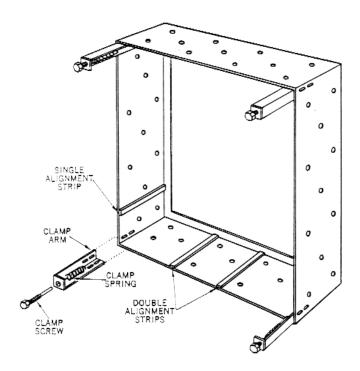
This constant pressure compensates for any set or deformation the gasket may experience after initial installation and ensures a constant seal at all times.
